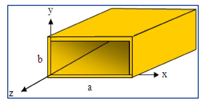
Dimensions of the waveguide which determines the operating frequency range
